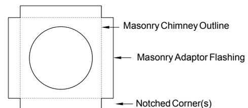
**FIGURE 31 Masonry Adapter Flashing Installation**
