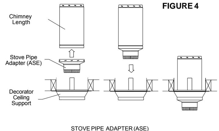
The crimped end (stub) of the Stove Pipe Adapter is intended to fit inside of the flue pipe from a solid fuel appliance, thus preventing condensate drips at the chimney connection.
