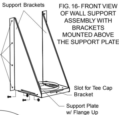
**FIG. 16- FRONT VIEW OF WALL SUPPORT ASSEMBLY WITH BRACKETS MOUNTED ABOVE THE SUPPORT PLATE**
