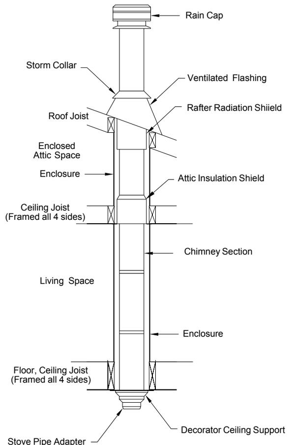
**FIGURE 6 Two Story Installation (Enclosed Attic)**
