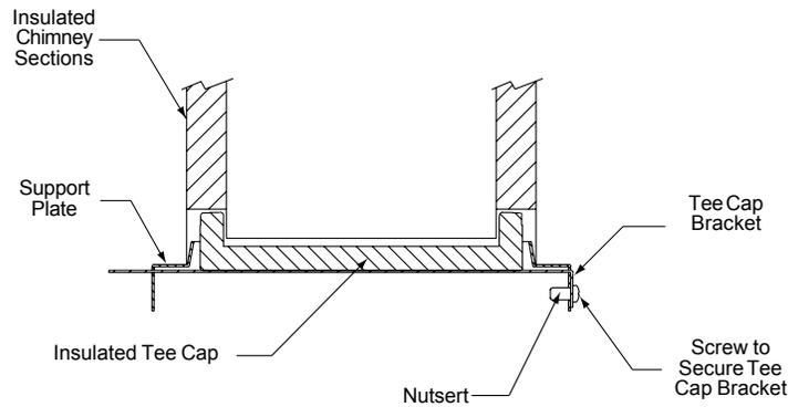
**FIGURE 15 - Securing of Insulated Tee Cap**
