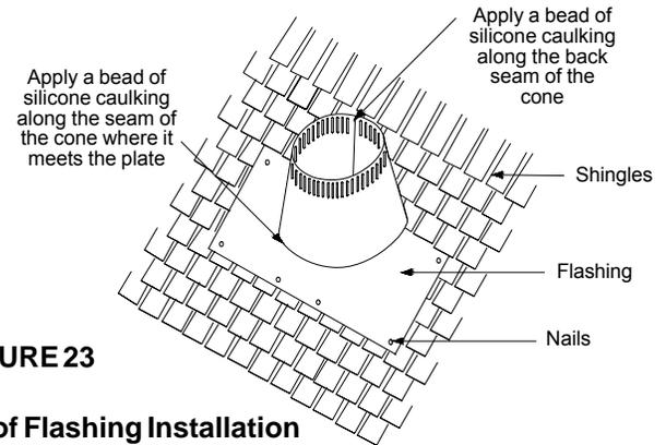
**FIGURE 23** Roof Flashing Installation
